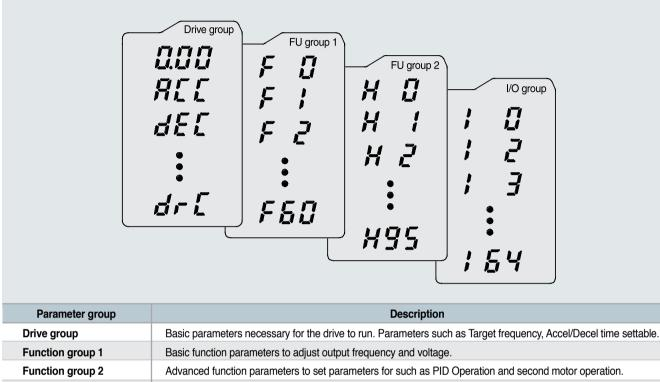
I/O (Input/Output) group Parameters necessary to make up a sequence using multi-function input/output terminal.
